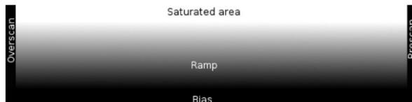
Figure 1: Example of a TDI image taken with the ESO test bench. Here is a 2148x512 pixels size image. A legend has been added. The area where is the ramp, is also called in this paper sensitive area.
