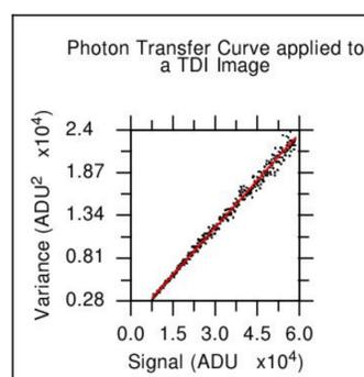
Figure 4: Example of a photon transfer curve realized with two TDI images. Similar pattern is observed with the technique based on one TDI image.
