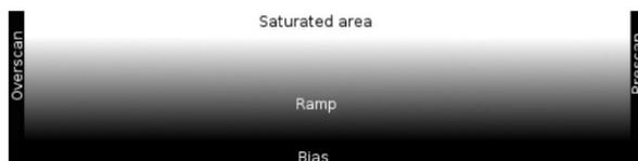
Figure 1: Example of a TDI image taken with the ESO test bench. Here is a 2148x512 pixels size image. A legend has been added. The area where is the ramp, is also called in this paper sensitive area.
