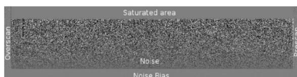
Figure 3: Example of noise pattern after subtraction of two images. Similar patterns are observed with same characteristics when we apply the pixel to pixel subtraction (Method two).
